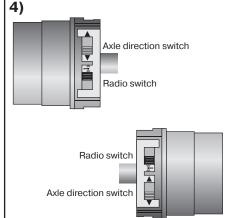
If the shutter moves in the wrong direction, the axle direction has to be changed. This is done as follows:
