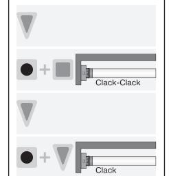
First press and hold the learn button. Within 3 seconds also press the DOWN button for the lower limit or the UP button for the upper limit position and hold both buttons.
