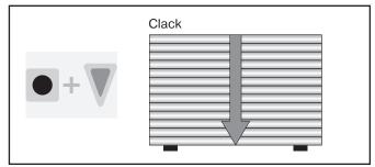
Travel to the desired upper end limit position. Subsequently press the learn button and the UP button until the tubular drive makes a "clack" sound.
