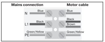
The brown wire and black wire are connected together at "L".
