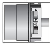
Slide the radio switch to position  $\P$  . (The tubular drive goes into learn mode for 3 minutes).
